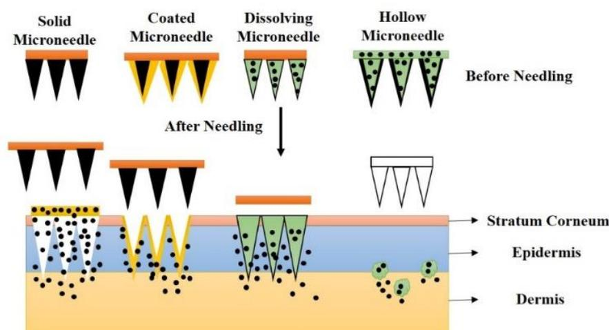
**Figure 2:** Different types of microneedles on skin layer
