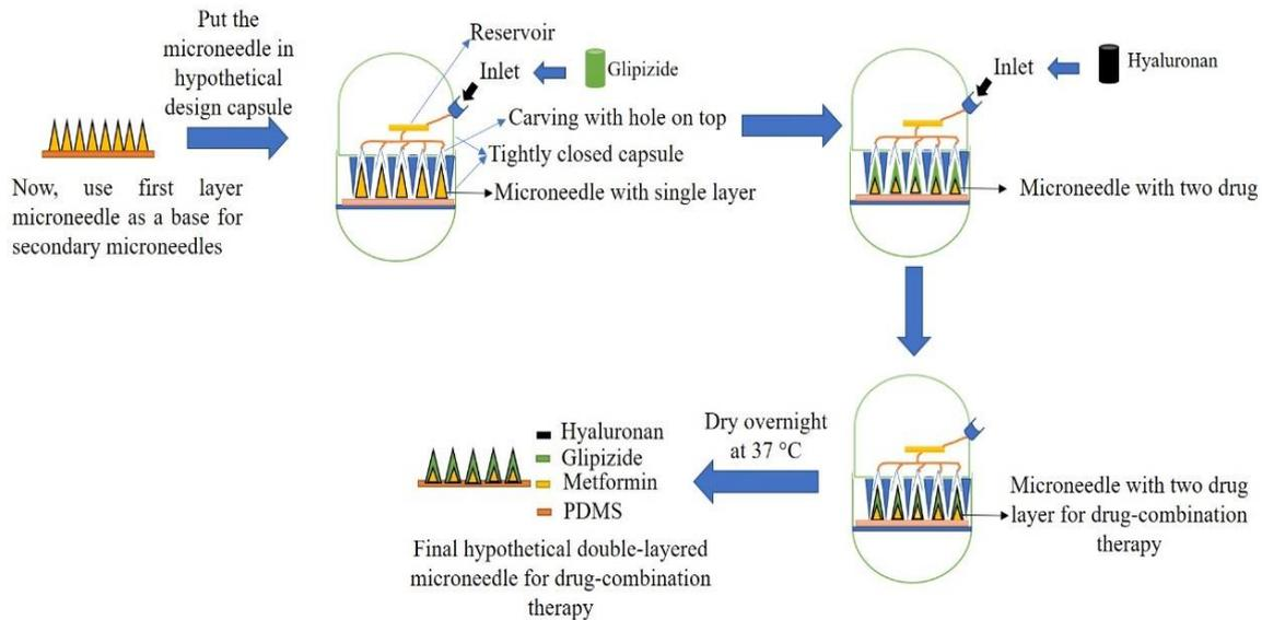
**Figure 6:** Preparation of double layer dissolving microneedle
