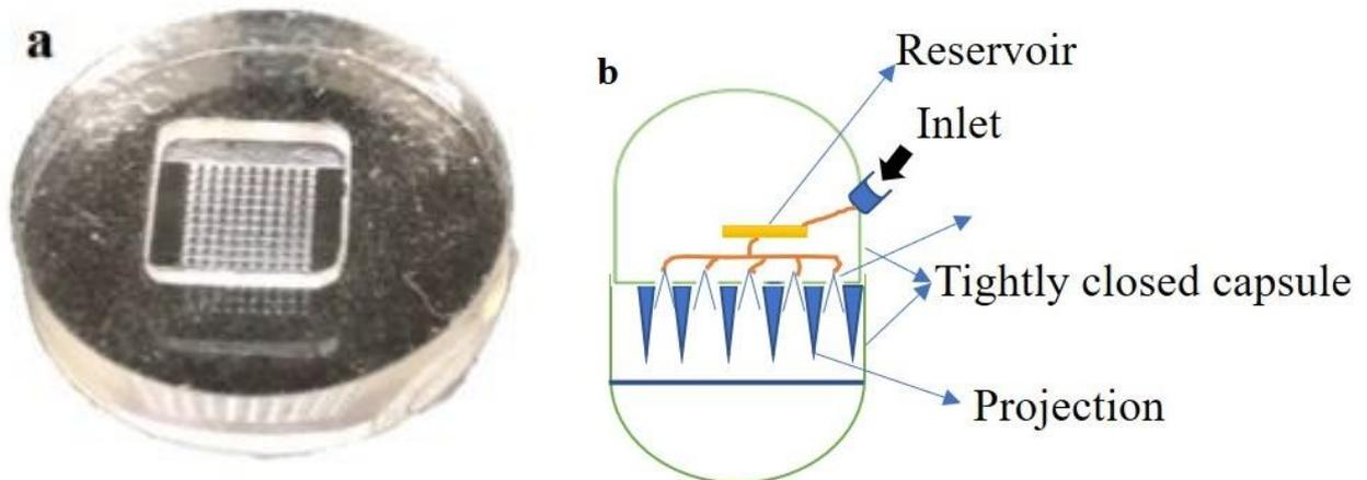
**Figure 4:** a: Primary mould used to form first-layer microneedle, b: Hypothetical-design capsule for developing double-layer microneedles.
