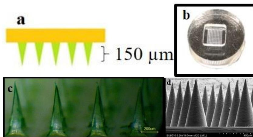
**Figure 1:** a. Basic Structure of Microneedle, b. Microneedle mould, c. Bright field micrographs of dissolving Microneedle, d. SEM image of Microneedle[4]
