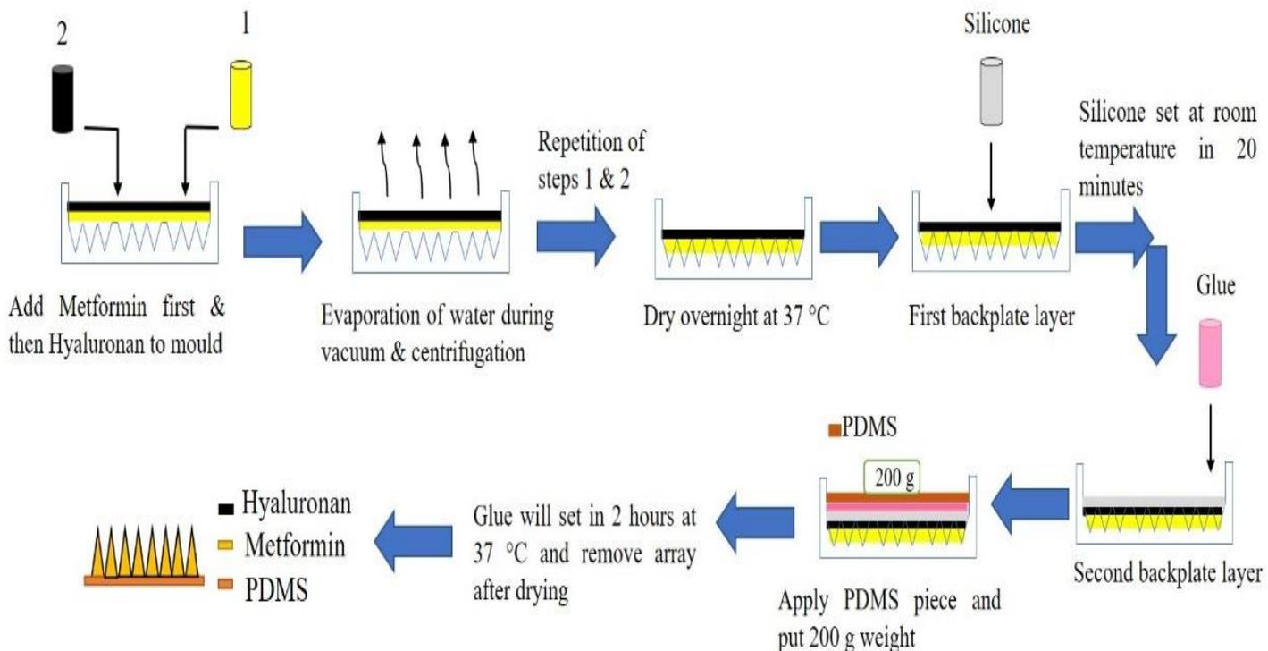
**Figure 5:** Preparation of single layer dissolving microneedle [18]
